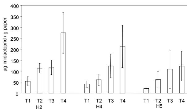
**Figure 1.** Quantity of imidacloprid ( $\mu\text{g/g}$ ) found in paper filters in the considered exposure times for the three Gaucho<sup>®</sup> dressed corn hybrids (mean  $\pm$  S.D.).
